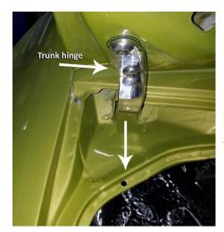
2) Locate and mark a spot in the center of the weather strip channel, directly across from the center of the trunk hinge as shown. Drill 1/4" hole at the mark.
