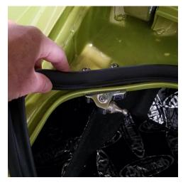
1) Apply anti-seize to a  $1/4^{"}$  X  $3/4^{"}$  socket cap flathead bolt and loosely fasten the "L" bracket into the hole in the outer corner of the Upper Strut Mount as shown.
