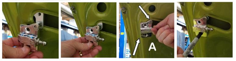
2.) "Hook" the "L" bracket into the top pocket in the deck lid. Slide the bracket until it contacts the inside edge of the top corner of the pocket and the bracket is parallel to the outer edge of the seam on the deck lid (Image A). Once in position, mark the two holes for drilling.
