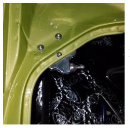
4.) From the underside of the drip rail, use the lower strut mount as a template and drill the additional two 5/16'' mounting holes. Apply antiseize to the  $5/16'' \times 3/4''$  button head bolt and fasten the bracket permanently.
